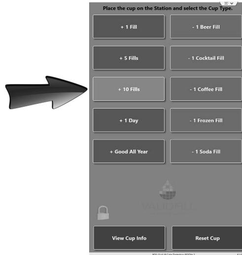
Once the cup has been successfully programmed you will see a Pop-up message that says, "The Cup has been Successfully Programmed." If you receive an error message ensure the cup has a tag that is properly installed and valid for the location.
