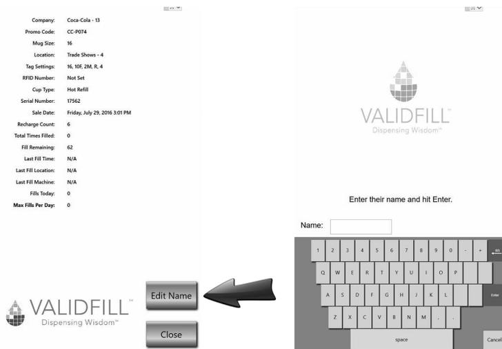
To add or edit the name place the cup on the puck and open the cup info screen. Touch the designated button which will launch the Keyboard. Type in the name touch the Enter Key to save the name to the cup. Use the same steps to edit a cup.
