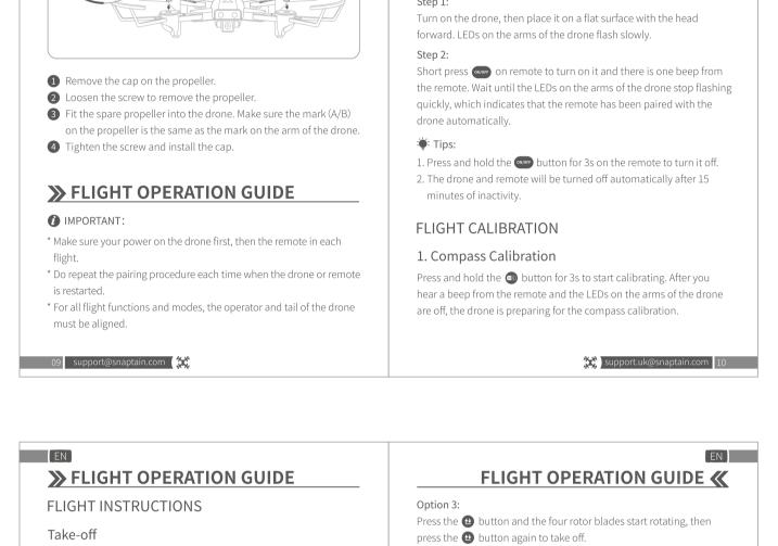
PAIR THE REMOTE WITH THE DRONE
