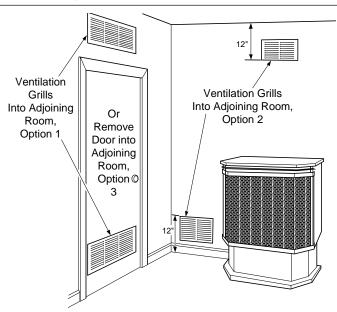
Figure 4 - Ventilation Air from Inside Building
