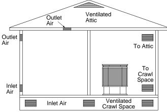
Figure 5 - Ventilation Air from Outdoors
