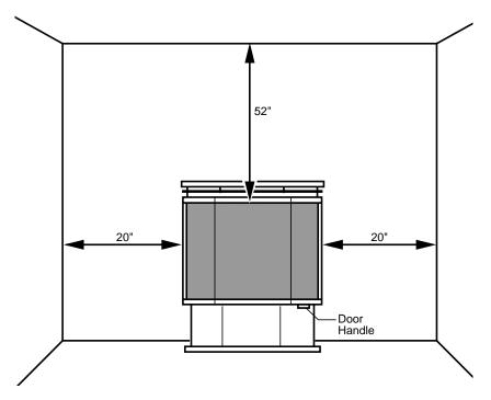
Figure 7 - Minimum Clearance to Wall and Ceiling
