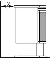
Figure 6 - Minimum Clearance to Back Wall
