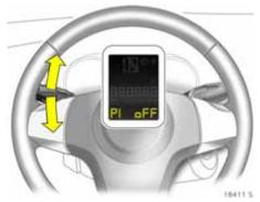
push the turn signal stalk (left) up or down and select the desired function P1 - P7 - see the table on the next page,
