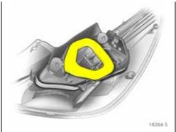
9. Ensure that the bulb holder seal is positioned as illustrated.
