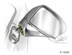
For the safety of pedestrians, the exterior mirrors of the Corsa VXR are released from the holder if they are bumped. Fit mirror housing to holder with latching lugs and engage by striking gently.
