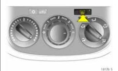
Heated rear window, heated exterior mirrors \*:
