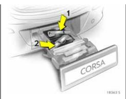
Fold in the bulb holders on the backs of the tail lights.
