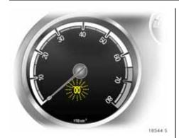
If the diesel particle filter needs cleaning and recent driving situations did not allow the function to automatically operate, then control indicator  $\mathfrak{W}$  will flash. If this occurs, then you may continue to drive the vehicle normally. The vehicle will not be damaged and does not require service.
