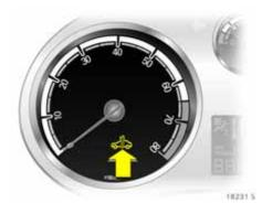
Control indicator for immobiliser औ Control indicator औ illuminates briefly when the ignition is switched on.
