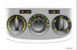
The buttons for cooling ‡ and air recirculation ♠ are only found on versions with air conditioning system ♣.
