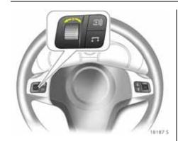
Selection using left adjuster wheel on steering wheel \*: Rotate and press knurled wheel.
