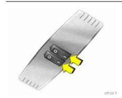
Courtesy lights and rear reading lights & Centre switch position: rear interior light illuminates together with the front one.
