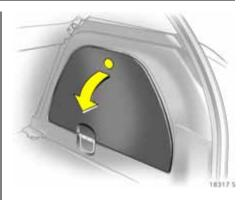
The tyre repair kit is located in the right-hand compartment of the luggage compartment.
