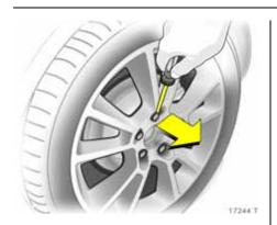
Alloy wheels **\***: Disengage the wheel bolt caps with a screwdriver and remove. Protect the wheel by inserting a soft cloth between the screwdriver and alloy wheel.
