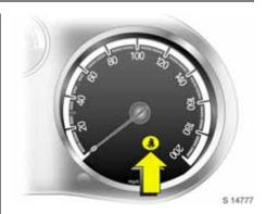
Control indicator \$\frac{4}{2}\$ indicating that driver's seat belt has not been fastened When the ignition is switched on, control indicator \$\frac{4}{2}\$ illuminates for approx.
