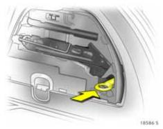
The towing eye is located in a recess.
