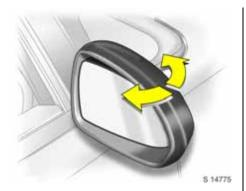
For the safety of pedestrians, the exterior mirrors will swing out of their normal mounting position if they are bumped with sufficient force. Reposition the mirror by applying slight pressure to the mirror housing.
