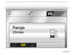
If less than 30 miles (50 km) can be driven with the fuel in the tank, the warning "Range" appears on the display.
