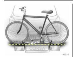
Place the wheel recesses such that the bicycle is more or less horizontal. Here, the distance between the pedals and the tailgate should be at least 5 cm. Setting the wheel recesses – see page 190.
