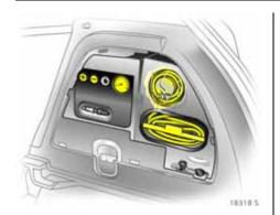
1. Remove the sealant bottle and holder with the air tube from the compartment.
