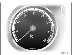
Control indicator  $\mathfrak{W}$  extinguishes as soon as the self-cleaning operation is complete.
