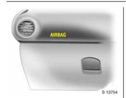
The front passenger's seat front airbag system can be recognised by the word **AIRBAG** above the glove compartment.
