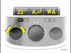
Set automatic mode on Electronic Climate Control system \*: Press AUTO, preselect temperature with rotary knob, open air vents
