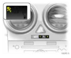
In the event of a fault in the airbag systems, the LEDs flash in button % for deactivation of the front passenger's airbag systems, and control indicator 2 also illuminates in the odometer display.
