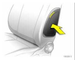
The side airbag system **\*** is identified by the covers on the outboard sides of the front seat backrests.
