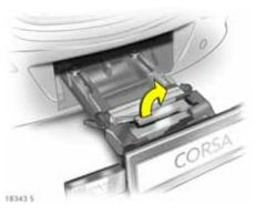
Unfold pedal crank recesses Fold one or both pedal crank recesses upwards until the diagonal support engages.
