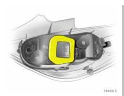
9. Ensure that the bulb holder seal is positioned as illustrated. Fit the round seal on the fastening bolt.
