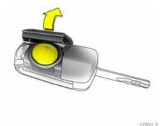
Remote control battery replacement Replace the battery as soon as the range of the remote control begins to shrink.
