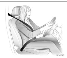
Adjust height such that the seat belt passes over the shoulder and rests against the shoulder. It must not pass over the neck or upper arm.
