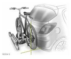
Align the bicycle in the longitudinal direction of the vehicle: Slightly loosen the pedal bearing mount - see page 189, Fig. S 14629.
