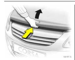
There is a safety catch on the underside of the bonnet: lift this upwards and open the
