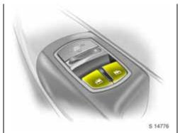
Operation with two switches in the driver's door armrest for the front windows. Additional switch in the front passenger's door.
