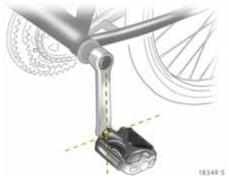
Prepare the bicycle for attachment Rotate the left pedal (opposite the chain cog) vertically downwards. The pedal on the left pedal crank must be horizontal.
