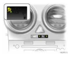
The airbag systems for the front passenger's seat are now deactivated. To indicate this, both LEDs in button 2 and control indicator 2 in the odometer display remain illuminated when the ignition is on.
