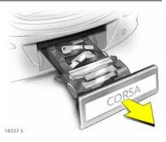
Completely pull out the Flex-Fix system until you hear it engage.
