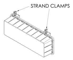
Note that if the strand mount option is selected for the radio along with internal antenna, the radio **must** be mounted horizontally on the strand as shown.
