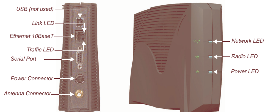
Figure 41 EUM3000 LEDs and Connectors
