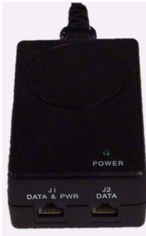
Figure 7 PoE Injector - Data & PWR and Data Ports
