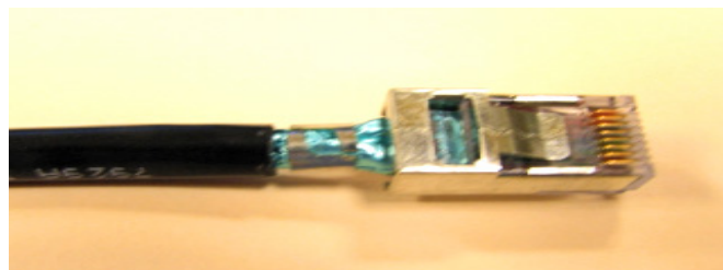
Figure A-9 Assembled cable terminating end
