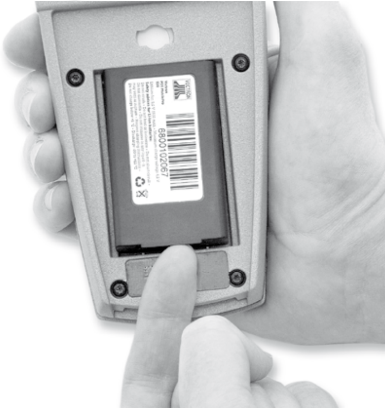
Fig. 8: Lifting the battery
