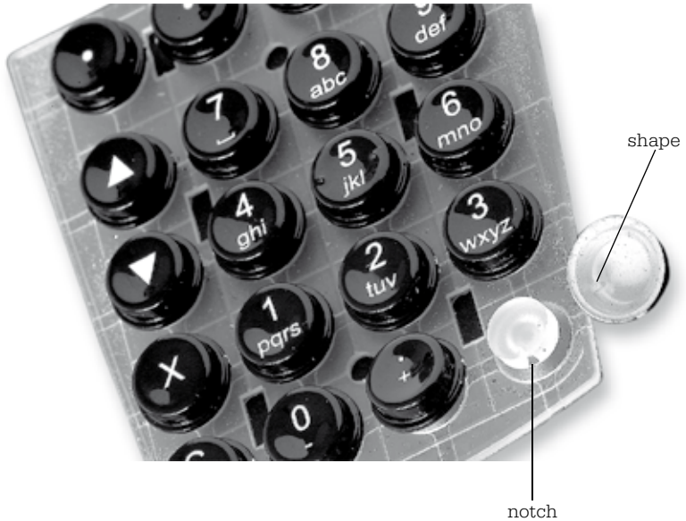
Fig. 28: Putting on the key caps
