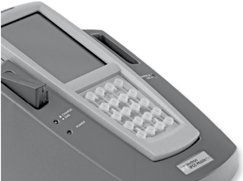
Fig. 27: Unremovable keyboard pad
