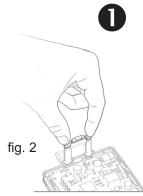
With the thermostat removed from the backplate, insert the Skyport Key. Install the Locking Clip as shown in figure 2.
