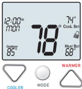
To **unlock** the keypad, press and hold the **MODE** button. While holding the **MODE** button, press the **WARMER** and **COOLER** buttons together.
