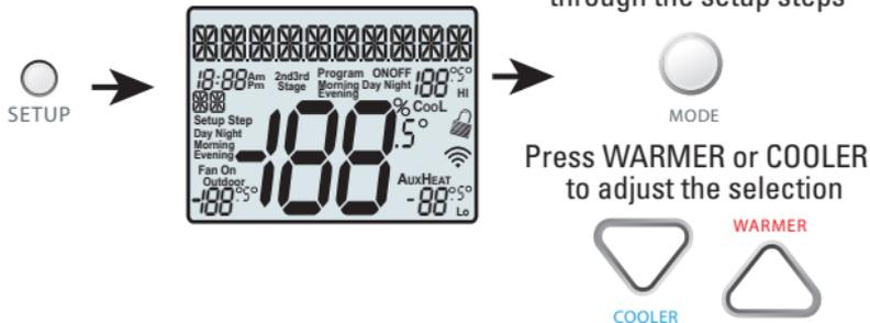
**Technician Setup is for diagnostic and testing purposes and is intended for use by a qualified technician. See page 15 for more detailed instructions.**
