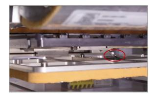
Newer ovens have delicate switch sensors. If the tray is not properly lifted off of this sensor, it can be damaged.
