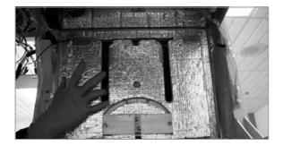
**2** Open the slide dryer, reaching through the elevator door to grasp the slide dryer door.
