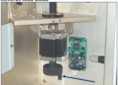
If the Transport Table is blocking the Elevator Hand Crank, turn the Elevator Lead Screw by hand.
