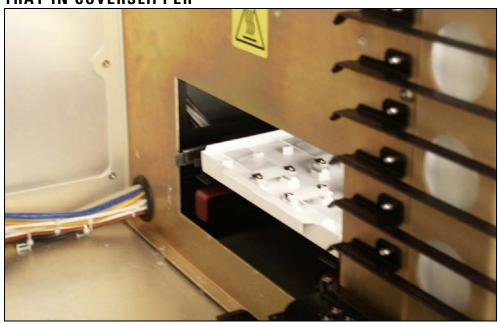
BRACKETS PULLED OUT BEFORE REMOVING TRAY
