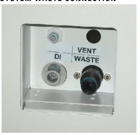
The best way to plumb the system is using a dishwasher tailpiece between the trap and the wall of the facility. The tailpiece must be 3/8" OD (outside diameter) with an HB (hose barb) connection on it.
