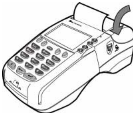
Figure 8 Closing Paper Roll Cover
