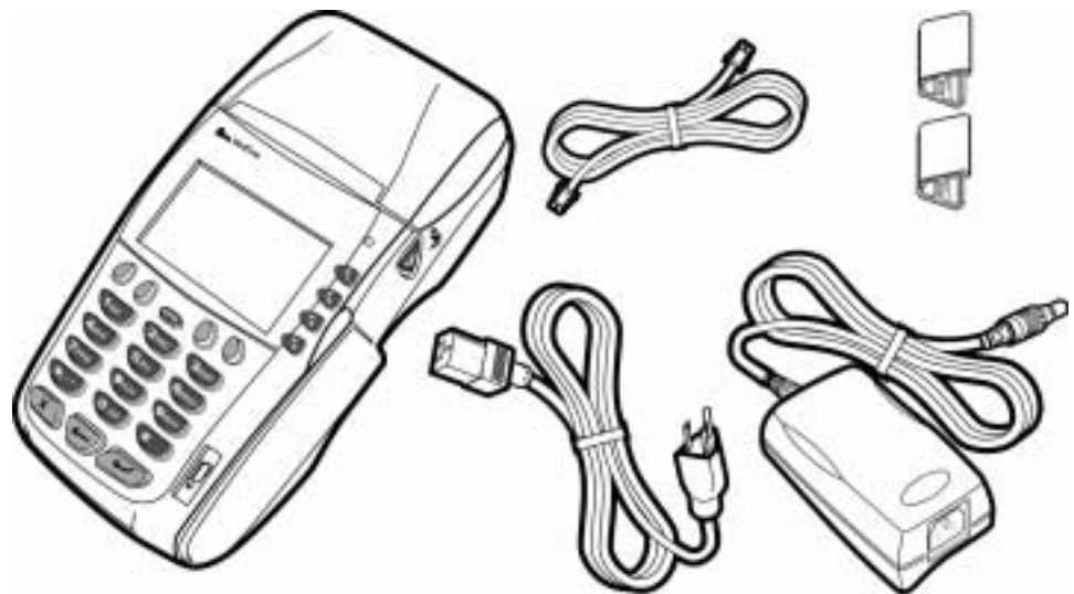
Figure 1 Omni 37xx Product Components
