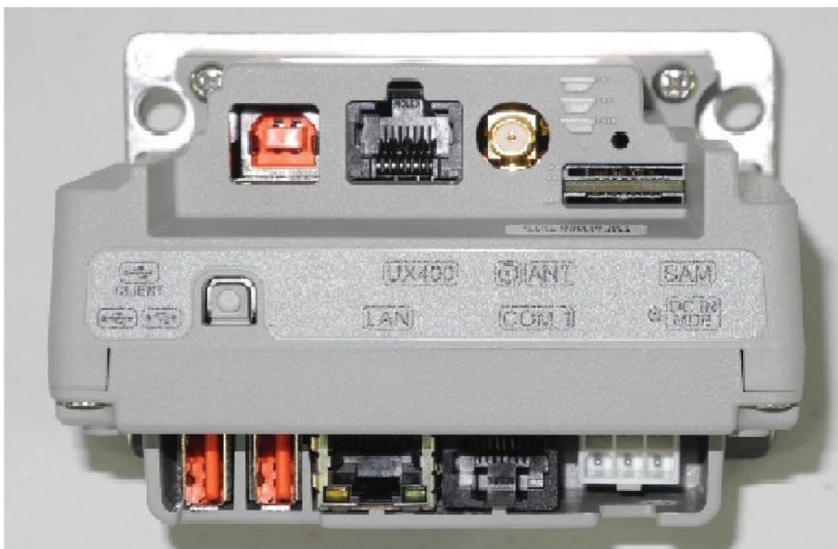
UX301 Underside View
