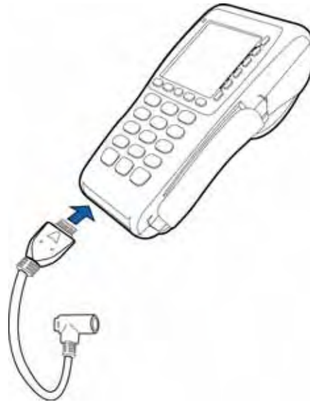
Figure 4 Power Adapter Cable Connection to a V x 670 Terminal
