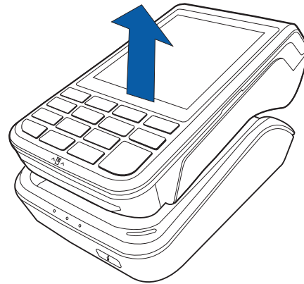
Figure 16 Undocking the Terminal from the Base
