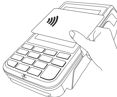
Figure 24 Contactless Smart Card Transaction
