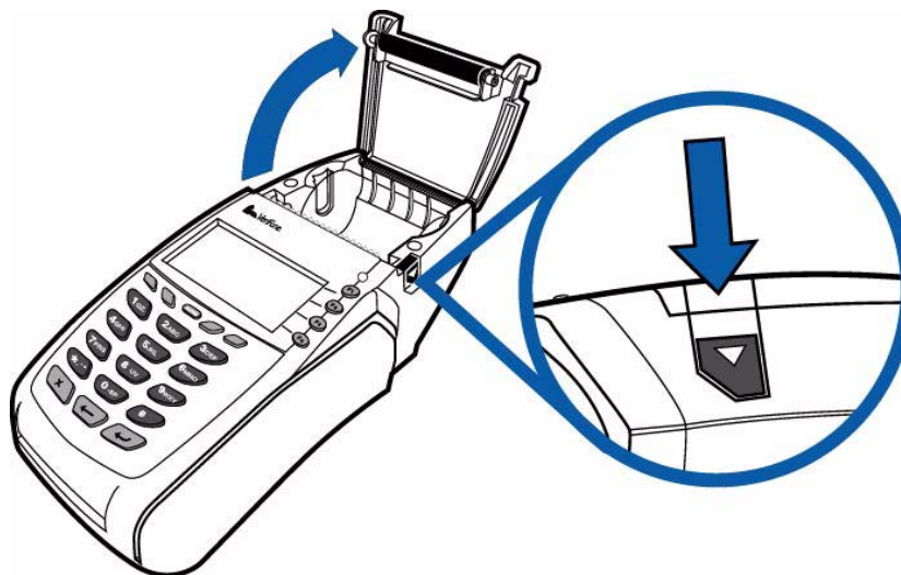
Figure 7 Opening the Printer Cover
