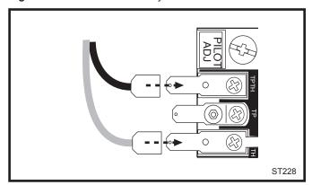
Fig. 43 Attach switch wires to valve.
