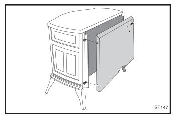
Fig. 15 Remove rear shroud.
