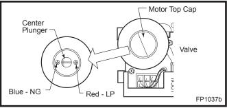
Fig. 62 Depress and turn center plunger.
