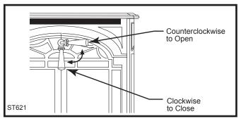
Fig. 44 To open the front doors, turn handle counterclockwise.
