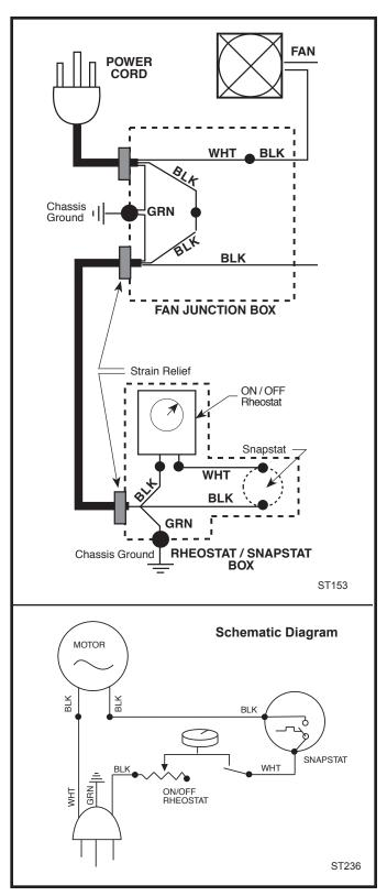
Fig. 70 Fan circuit.
