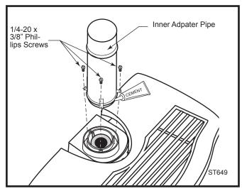
Fig. 22 Simpson DuraVent - install inner adpater pipe.
