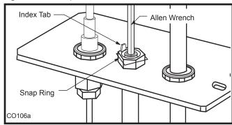
Fig. 57 Remove pilot orifice.
