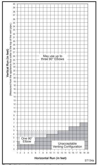
Fig. 7 Horizontal vent termination window.
