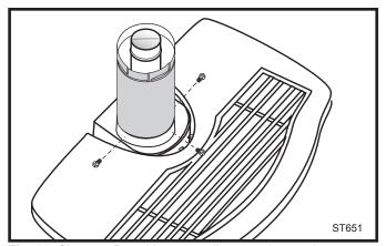
Fig. 23 Simpson Dura-Vent - install outer adapter pipe.
