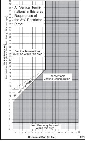
Fig. 8 Vertical vent termination window.
