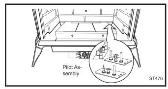
Fig. 46 Pilot Assembly location.
