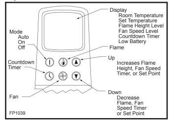
Fig. 50 Transmitter diagram.
