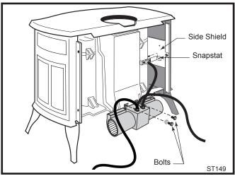
Fig. 16 Attach blower assembly and snapstat.
