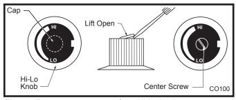
Fig. 55 Remove center screw from Hi-Lo knob.
