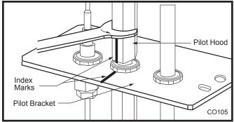
Fig. 60 Remove pilot hood. (Your pilot may have a different
