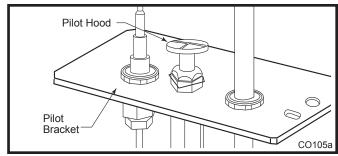
Fig. 58 Remove pilot hood.
