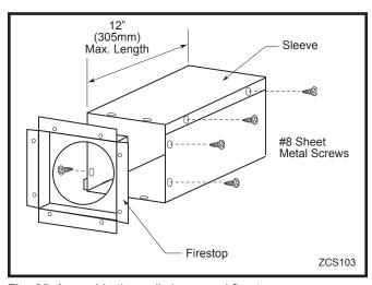
Fig. 25 Assemble the wall sleeve and firestop.
