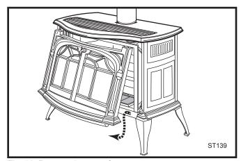
Fig. 36 Remove the stove front.
