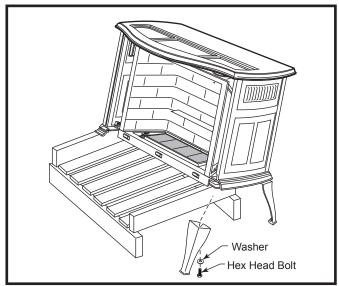
**Fig. 13** Carefully tip stove onto back legs. Leave pallet under stove to keep stove from falling fully forward.
