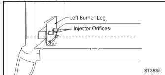
Fig. 63 Remove and replace injector orifices.
