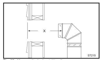
Fig. 27 Measure the horizontal length.
