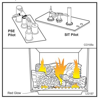
Fig. 48 Correct pilot and burner flame patterns.
