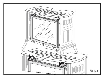
Fig. 37 Release the latches to remvoe the glass frame.
