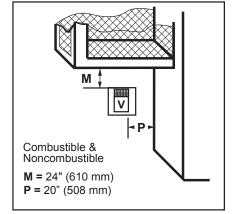
\*NOTE: Termination in an alcove space (spaces open only on one side and with an overhang) is permitted with the dimensions specified for vinyl or non-vinyl siding and soffits. 1. There must be a 3' (914 mm) minimum between termination caps. 2. All mechanical air intakes within 10' (1 m) of a termination cap must be a minimum of 3' (914 mm) below the termination cap. 3. All gravity air intakes within 3' (914 mm) of a termination cap must be a minimum of 1' (305 mm) below the termination cap.
