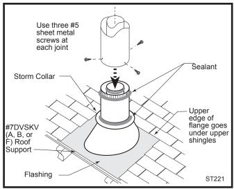
Fig. 33 Roof support and flashing.
