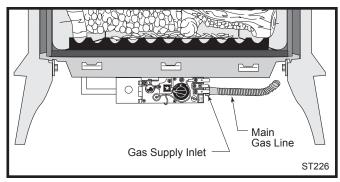
Fig. 52 Attach the gas line to the left side of the valve.
