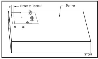
Fig. 54 Adjust air shutter according to Table 2.
