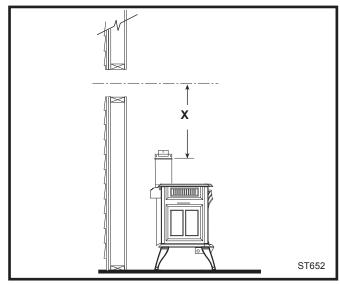
Fig. 26 Determine the vertical pipe length.
