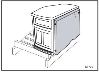
**Fig. 12** Slide stove back just far enough to access rear leg holes.
