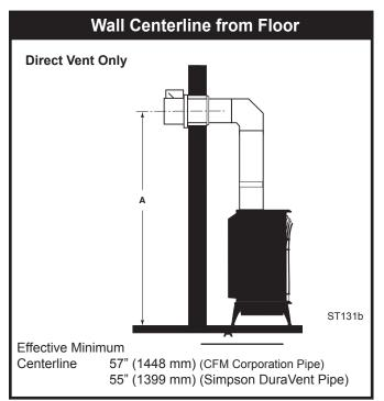
Fig. 5 Minimum wall centerline.
