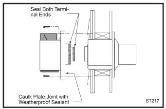
Fig. 29 Install the vent terminal.
