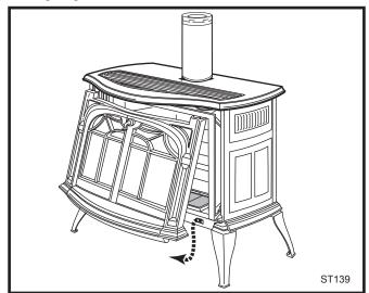
Fig. 64 Remove the Stove Front.
