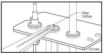
Fig. 61 Remove pilot orifice.
