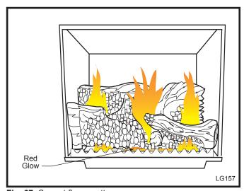
Fig. 67 Correct flame pattern.
