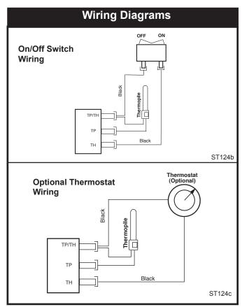
Fig. 68 On/off switch and optional thermostat circuit.
