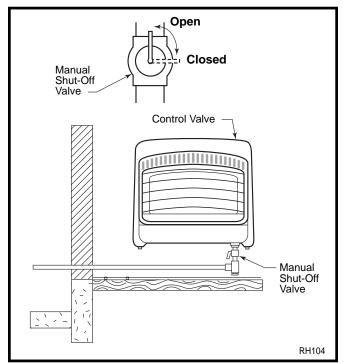
Fig. 7 Manual shut-off valve location.
