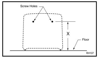
Fig. 5 Optional wall mounting screws for floor installation.
