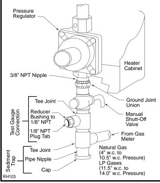
Fig. 6 Gas line connection.
