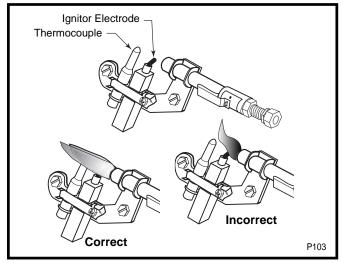
Fig. 9 Proper pilot flame.
