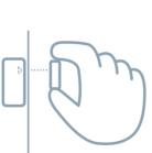
3. Hold the magnet up to the Versa, in the location you plan on mounting it.
