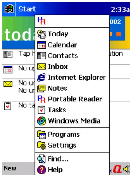
Figure 4.1-3 Mobile Reader Pull Down Menu Screen
