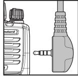
nector pin using the screws supplied with the Speaker/ Microphone. Hold the speaker grille up next to your ear while receiving. To transmit, press the **PTT** switch
