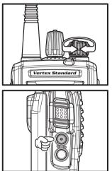
Press (or press and hold) the Programmable key again to quiet the noise and resume normal (quiet) monitoring.
