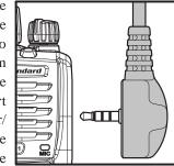
the plug using the screws supplied with the Speaker/ Microphone. Hold the speaker grille up next to your ear while receiving. To transmit, press the **PTT** switch on the Speaker/Microphone, just as you would on the main transceiver's body, and speak into the microphone on a normal voice level.
