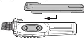
□ To remove the battery, turn the radio off and remove any protective cases. Slide the Battery Pack Latch on the bottom of the radio toward the front panel while sliding the battery down about 1/2 inch (1.5 cm). Then lift the battery out from the radio.
