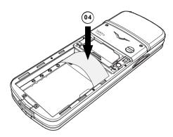
If you do not re-insert the battery or insert another battery immediately, insert the plastic placeholder (04) before replacing the back cover. This will make it easier to remove the back cover.
