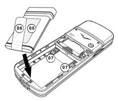
Insert the battery (05) bottom end first with the release tab (06) facing up from the rear of the phone. Ensure that the contacts on the top end of the battery align with the contact points (07) inside the battery compartment.
