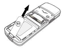
> Hold the release tab (03) and pull upwards to remove the battery from your Vertu phone.
