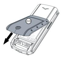
Turn the locking screw (02) a quarter of a turn anticlockwise, gently pivot (by no more than 45 degrees) and lift off the back cover (03) towards you as shown. If you accidentally remove the back cover while the phone is switched on, the phone will automatically switch off.
