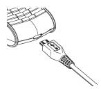
Insert the charger connector into the bottom of your Vertu phone as shown. Please ensure that the connector is inserted correctly, with the connector symbol uppermost.
