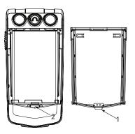
To replace the battery cover, carefully insert the internal clip(1) on the inside of the battery cover into the slot below the battery (2).
