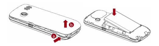
**Caution**: Install according to the illustration above to avoid breaking the battery connectors.
