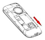
4) With the metallic contacts of the battery facing the metallic contacts in the battery slot, press the battery down until it locks into place, then fix its back cover.
