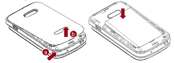
**Caution**: Install according to the illustration above to avoid breaking the battery connectors.
