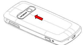
Pull out the top of the battery and remove.
