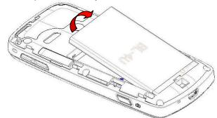
■ When installing the battery, insert the metal contact at the bottom of the battery into the corresponding slot of the mobile phone, and then press the battery down to install it in place. The battery must be ensured to be installed before power on.
