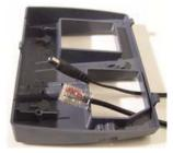
7. Attach the power cable and the RJ45 10-pin connector into the base of the 4500m unit. Make sure that the cables are routed into the channels.
