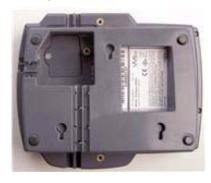
3. If you want to use any of the channels on the bottom of the 4500m unit, you need to remove the stand by depressing the spring clip on the wide side of the stand and lifting the stand off of the 4500m unit.
