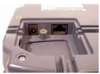
**Note:** Do not use 8-pin connectors as they can damage the jack. Use only ViVOtech-approved cables with 10-pin connectors.
