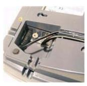
8. Reattach the stand if it was removed for routing the cables. Note that the stand helps to hold the cables in the channels.
