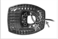
**Note:** The cable should always be positioned to the back of the ViVOpay 4800 - do not route the cable towards the front of the ViVOpay 4800.
