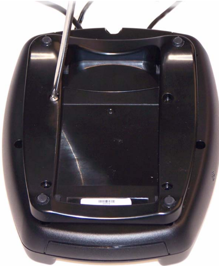
Figure 5. Attaching the wedge bracket
