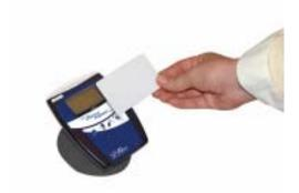
When a card/fob has been successfully read, an audible beep is emitted and four LEDs will be illuminated.
