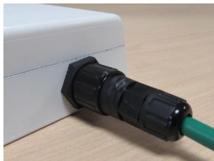
Figure 2-5. Cable Connector and Locking Collar
