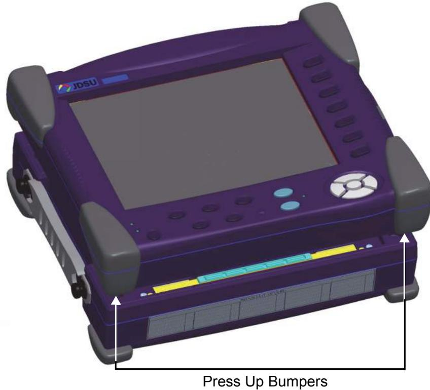
**IMPORTANT:** When lifting the base unit, be certain to apply force directly over the base unit mating connector (illustrated in [Figure 21 on page 30](#)). The lower bumpers are located on the front (display) panel of the base unit, and they are parallel with the mating connector provided on the bottom (connector) panel. In [Figure 40](#), the base unit mating connector is not visible; it is directly above the mating connector of the DMC.
