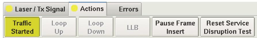
A blinking circle on a tab indicates that some action is required on your part. For example, if you are running a BERT test, the Actions tab may blink indicating that you need to start transmitting the BERT pattern.
