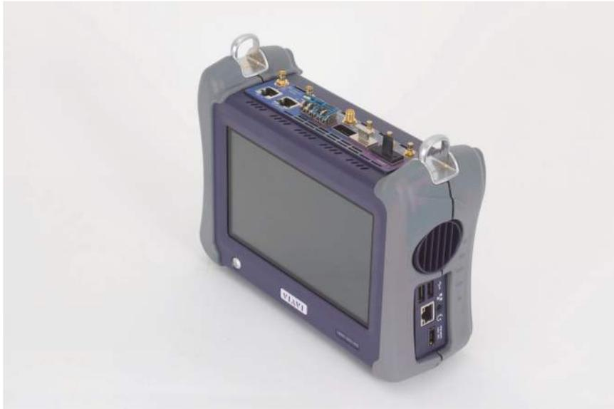
After selecting a test application, LEDs illuminate indicating which connectors to use for your test.
