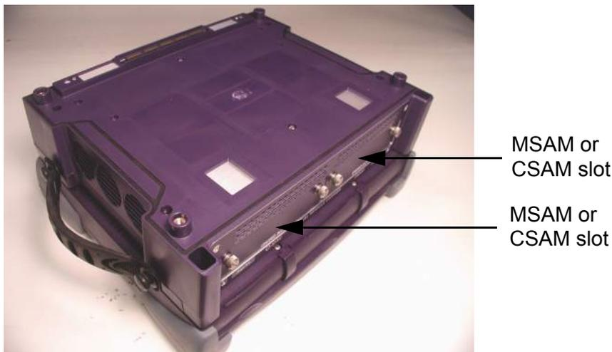
Figure 19 shows a DMC connected to a base unit. For assembly instructions, see [“Connecting a DMC to a base unit” on page 28.](#)
