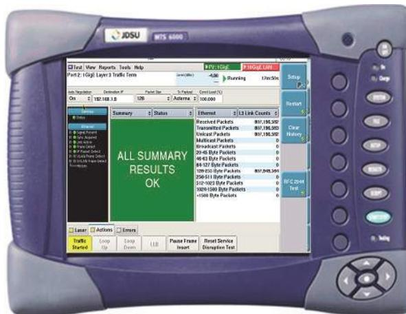
**Figure 11** T-BERD/MTS 6000AV2 with MSAM user interface
