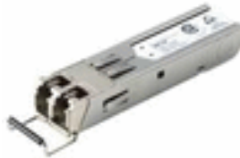
Figure 3 SFP transceiver with open bail-clasp latch
