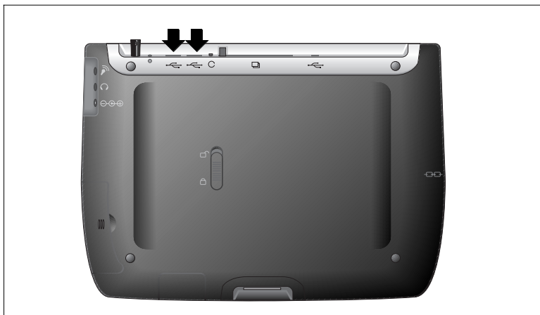
Figure 19: The External Keyboard/Mouse USB Ports
