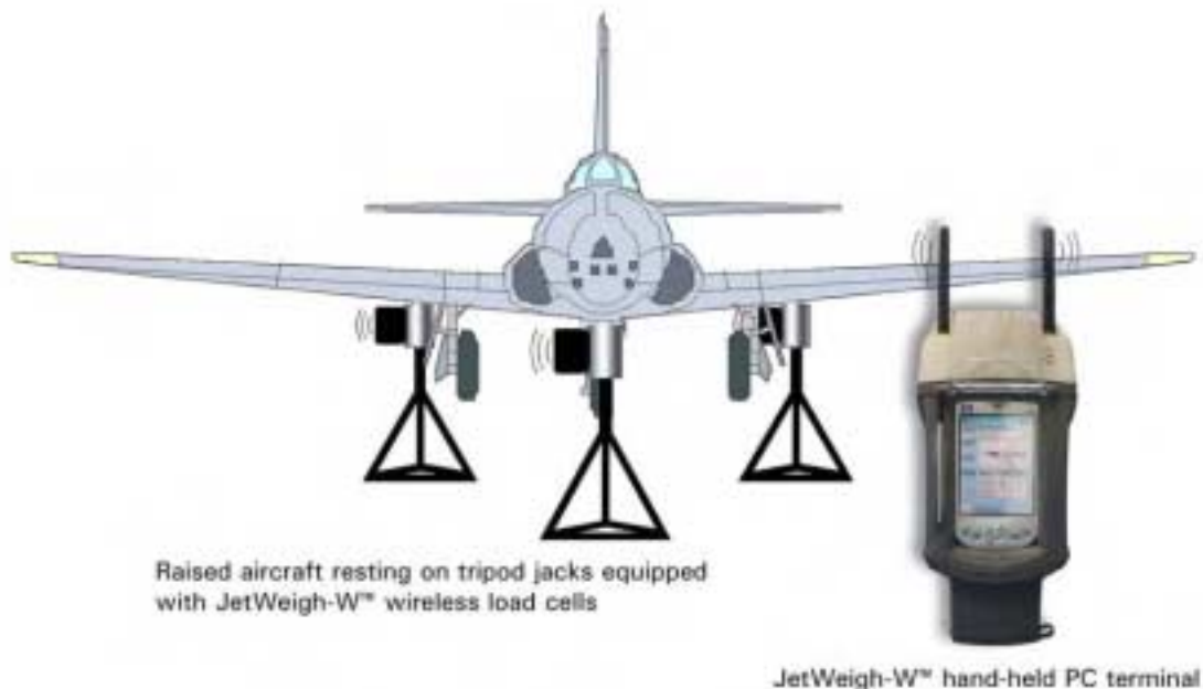
Figure 1-1. Typical JetWeigh-W™ Aircraft Weighing System
