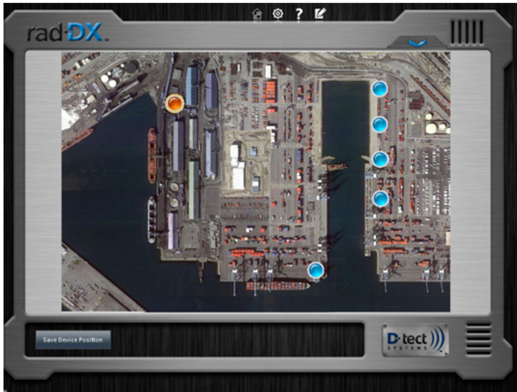
Figure 4: Application Home Screen with one alarming device icon and five normal device icons
