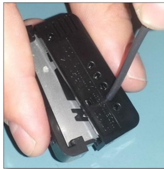
Figure 18 - Fiber optic cutter (Omron E39-F4)
