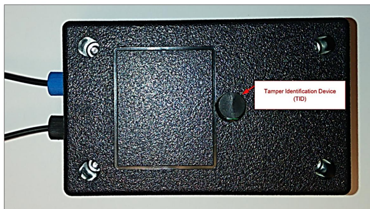
Figure 14 - Transmitter's Tamper Identification Device (TID)
