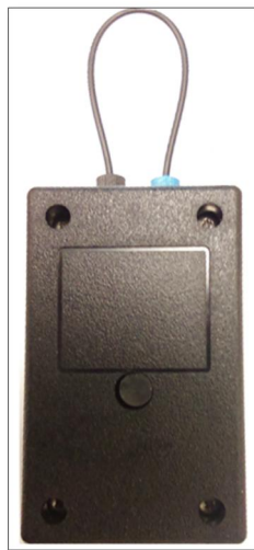
Figure 11 - Transmitter with fiber optic loop (back side)
