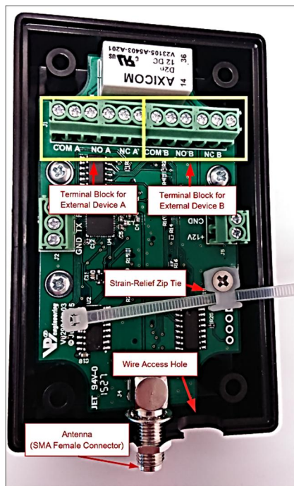
Figure 7 - Receiver's main terminal block, wire access point, zip tie for wires
