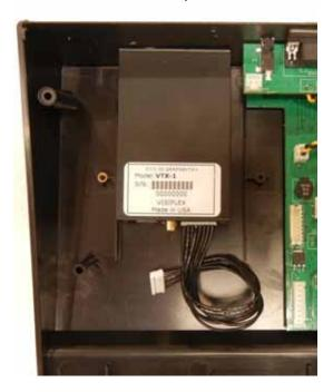
2. Secure the VTX-1 using the applicable bracket and connect the Data & Power Interface cable to the host product main board
