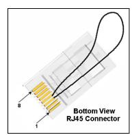
Should a dummy RJ45 dummy plug need to be made-up on site, ensure that the correct order of the wire used to short pins 3 & 4 is maintained as shown here.
