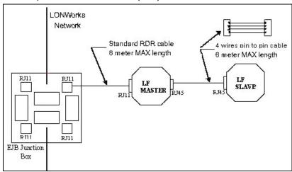
When the Master LF Exciter (from hardware Version C, Revision A-1) senses that the Slave has been disconnected, the Master audibly beeps continuously. To suppress the beeping, every Master is shipped with a dummy RJ45 (8P8C) male plug that shorts pins 3 & 4. The plug is typically found already inserted in the female Master/Slave RJ45 interface socket on the unit's main circuit board.
