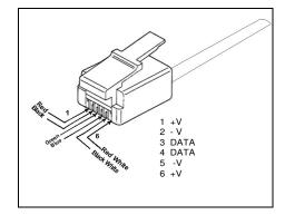
To wire a Master/Slave configuration, use an unshielded 4 conductor 26 AWG solid cable crimped at both ends with a RJ45 (8P8C) connector as illustrated below:
