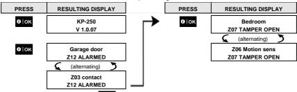
In response to additional clicking of the button, the display shows details of other events retained in open tamper (if any), or reverts to its initial state (see A above).
