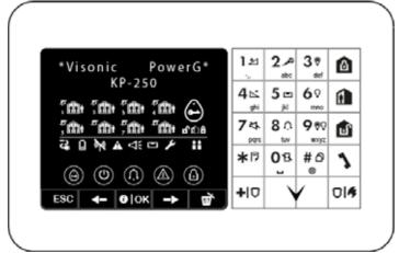
Note: The icons and numbers shown on the above keypad drawing are for illustrative purposes only. When executing a command, the KP-250 PG2 keypad's LED blinks red once to indicate transmission of the command to the control panel. If the operation is successfully completed, the green LED lights momentarily and a "happy tune" sounds. If the operation fails or cannot be completed, for example, when the system is "Not Ready", the red LED lights steadily and a "sad tune" sounds.
