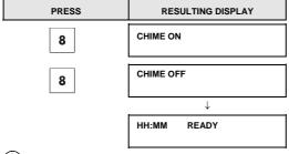
CHIME indicator lights steadily on the KP-250 PG2 keypad, when "chime on" is selected.
