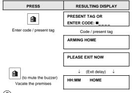
ARM indicator on both the KP-250 PG2 keypad and PowerMaster panel flashes during the armed state.
