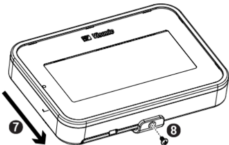
Figure 5 – Wall Mounting with External DC Cable
