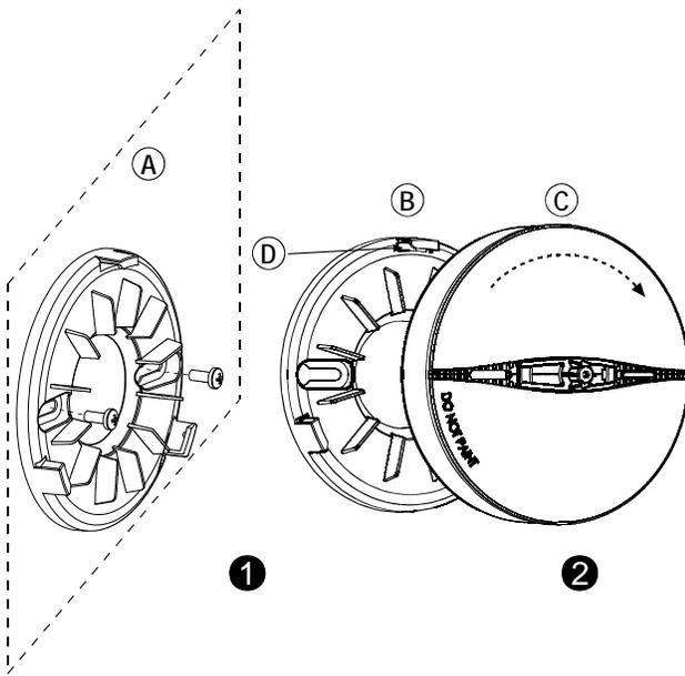
1. Mark and drill 2 holes in the mounting surface. Fasten the bracket to the mounting surface with 2 screws.
