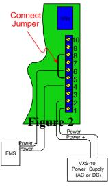
Use Separate power supplies for VXS-10 and EMS (normally open relay)
