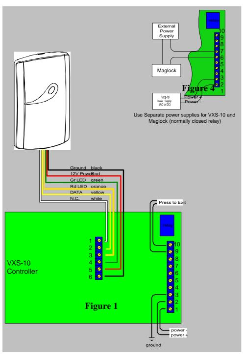
Connect EMS to VXS-10 Power Supply (AC or DC)
