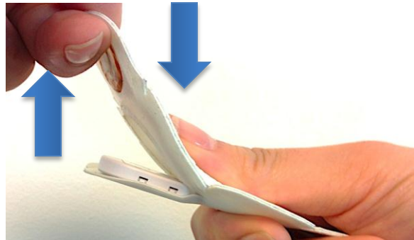
Figure 10: Pull the wing up while pushing thumb down on module side until sealed cavity is popped open and module is revealed. This hand gesture is similar to “popping” a pill or gum out of a foil packet.
