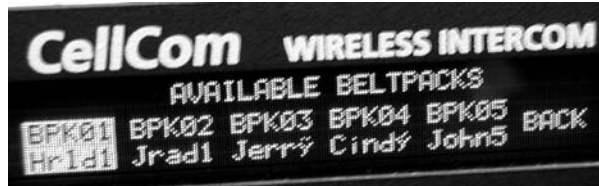
Figure 4: Scroll through the available beltpacks and push the rotary encoder to select
